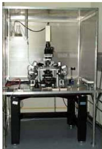
**Dr. Alon Korngreen** announces that the construction of the new multiple electrode recording setup funded by the Israel Science Foundation is complete. The new system allows simultaneous recording of ionic currents and membrane potential from two synaptically connected neurons or from two locations on the dendritic tree of a single neuron in brain tissue. These capabilities enhance our ability to investigate the computational properties of single neurons.
